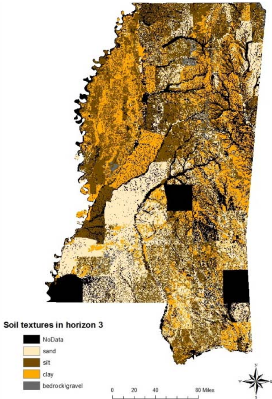
Figure 11 Generalized soil texture of H3 for map units across Mississippi derived from the Natural Resources Conservation Service (NRCS)'s Soil Survey Geographic (SSURGO) database.
