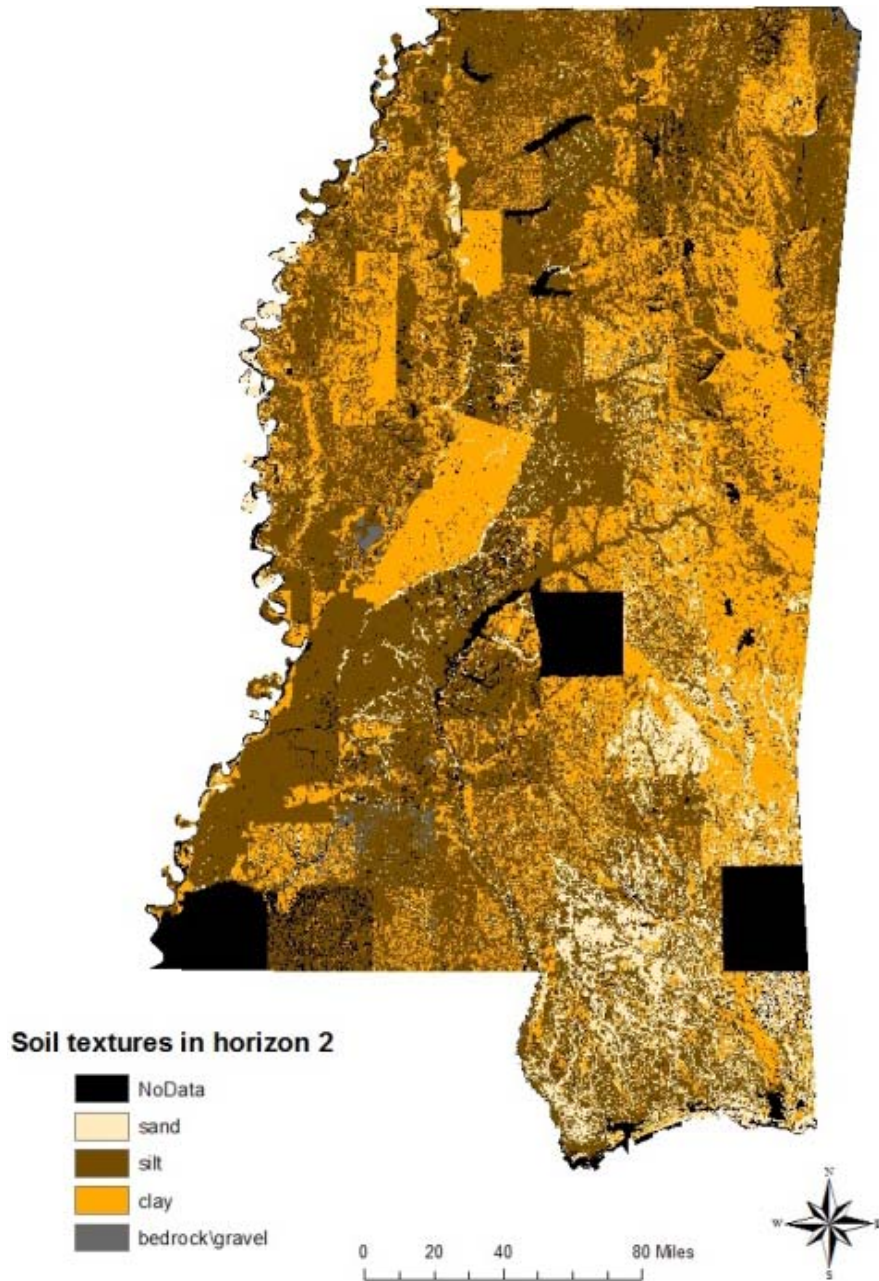
Figure 10 Generalized soil texture of H2 for map units across Mississippi derived from the Natural Resources Conservation Service (NRCS)'s Soil Survey Geographic (SSURGO) database
